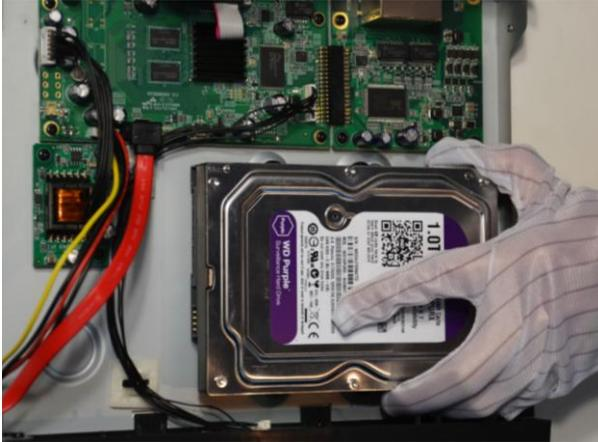
Step 4 Turn the device over, and fasten the rest two hard disk fixing screws, as shown in Figure 3-4.
