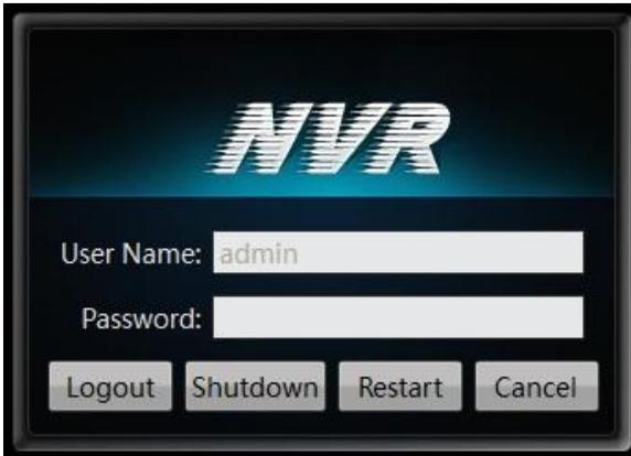
Enter the correct password and click **Shutdown**. When authentication is successful, the shutdown successful page is displayed, then cut off the power.
